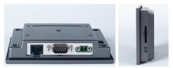
Figure 1.1 TPC-31T I/O Ports Arrangement
