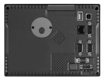
Figure 1.2 TPC-61T I/O Ports Arrangement
